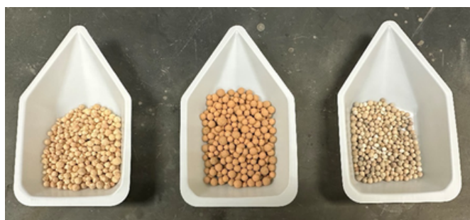
Figure 1. Visual representation images of the spent Claus catalysts. (A) spent Claus catalyst from gas plant A, (B) spent Claus catalyst from gas plant B, and (C) spent catalyst from gas plant C.
