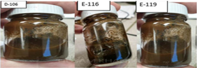
Figure 1. Sludge samples collected from D-106, HE-116, and HE-119 at the sulfur recovery unit of Plant J-87.
